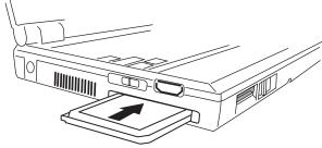
Sample inserting a PC Card
